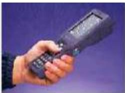
This is the DT-X10 which uses the same operating system and software as the IT3000, but has no printer. All options that apply to the IT3000 apply to this one in that scanners and card swipes can be incorporated.
